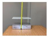
By adjusting the reflector upward from the bottom ridge of the base, which will sit on the floor of the flume directly under the level sensor, the flow meter will transmit and display the flow proportional to the simulated level. In this case a 24inch Parshall flume with the simulator set to 240mm can be verified against the chart on the next page. The flow on the transmitter should be comparable to 156.4 l/s.
