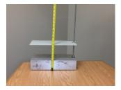
By adjusting the reflector upward from the bottom ridge of the base, which will sit on the floor of the flume directly under the level sensor, the flow meter will transmit and display the flow proportional to the simulated level. In this case a 24inch Parshall flume with the simulator set to 240mm can be verified against the chart on the next page. The flow on the transmitter should be comparable to 156.4 l/s.
