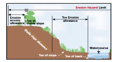
The toe erosion allowance is the setback that ensures safety if the toe of the slope adjacent to the watercourse erodes and weakens the bank, thereby increasing the risk of slope failure.
