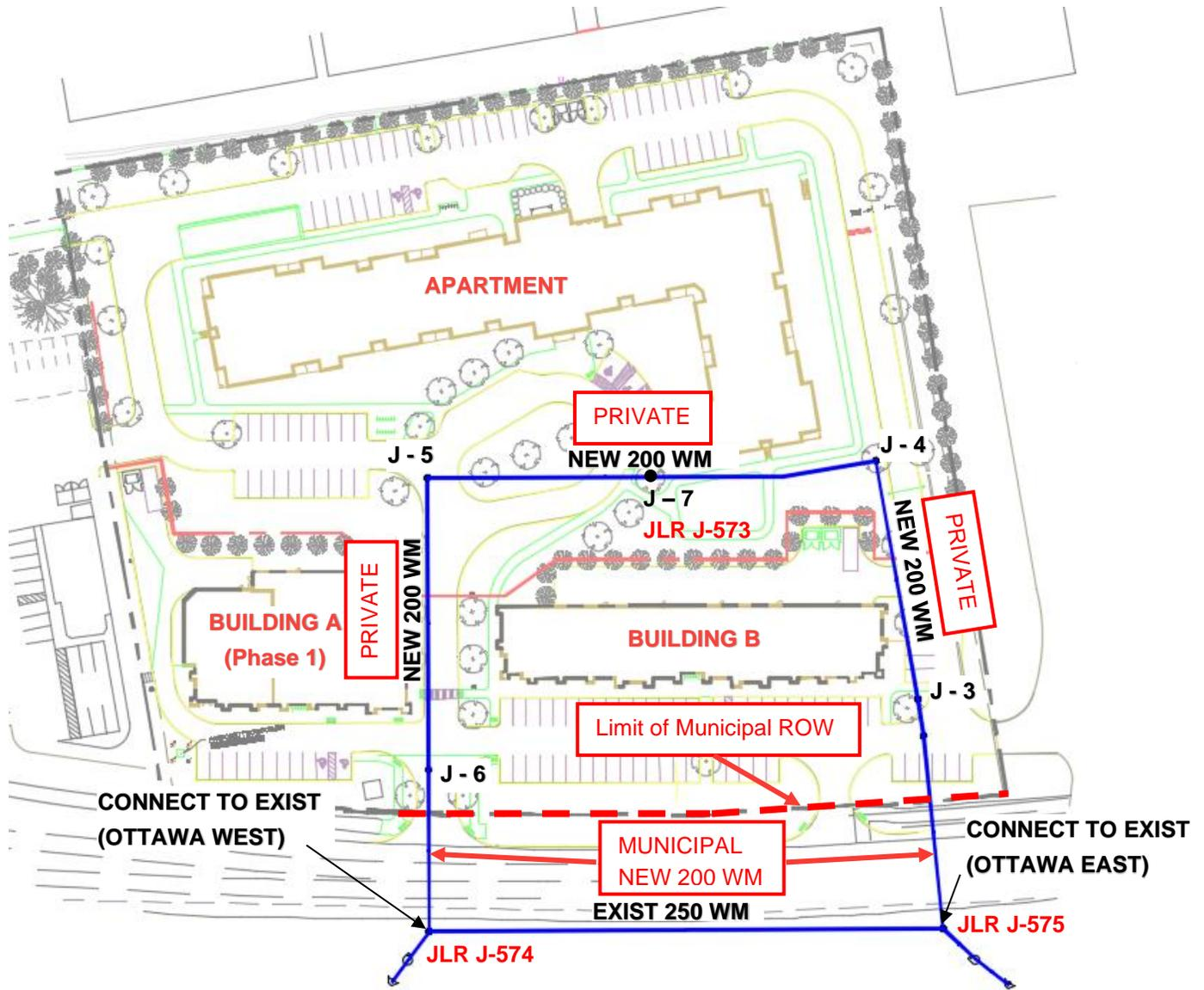
Figure 2.1: Water Distribution Model Schematic
