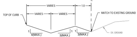
A.A C01 PROPOSED DITCH SECTION SCALE: NTS
