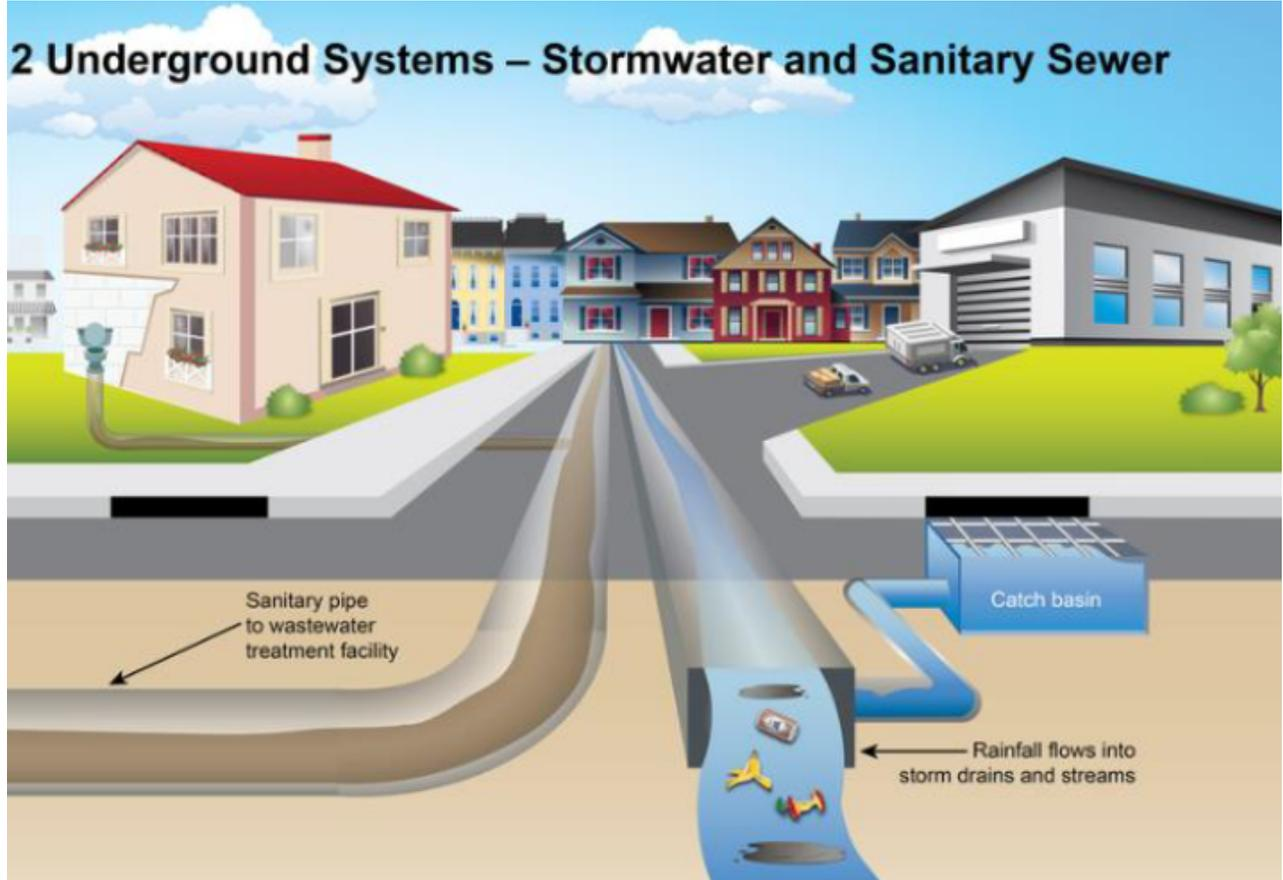
**Figure 3: Typical service connection in Mississippi Mills.**
