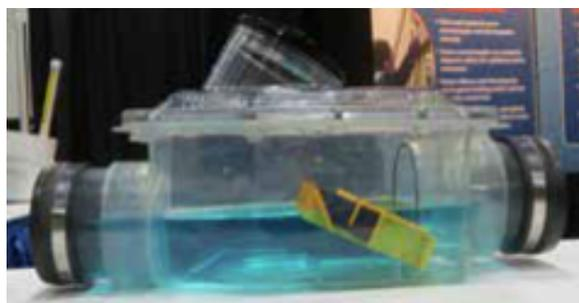
Example of a vented backwater valve.
