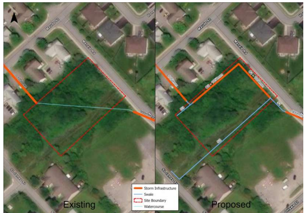
Figure 1: Existing and proposed drain alignment
