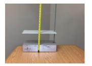
By adjusting the reflector upward from the bottom ridge of the base, which will sit on the floor of the flume directly under the level sensor, the flow meter will transmit and display the flow proportional to the simulated level. In this case a 24inch Parshall flume with the simulator set to 240mm can be verified against the chart on the next page. The flow on the transmitter should be comparable to 156.4 l/s.
