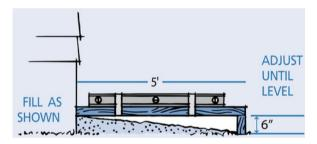
Place the long end of your slope gauge against the basement wall and the shorter end on the ground. The horizontal board should be level. If it is not, add soil at the basement wall until the level is achieved.
