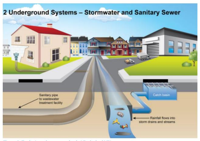
Figure 3: Typical service connection in Mississippi Mills.
