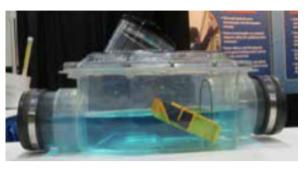
Example of a vented backwater valve.
