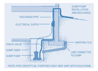
If you test the pump and it is not working properly:
