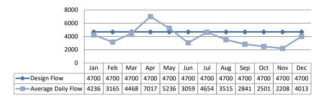
The flow spikes are associated to wet weather events such as rain and seasonal changes such as the spring snow melt.
