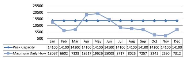
Note: Elevated flows above the peak capacity are directly related to snow melt and wet weather events.
